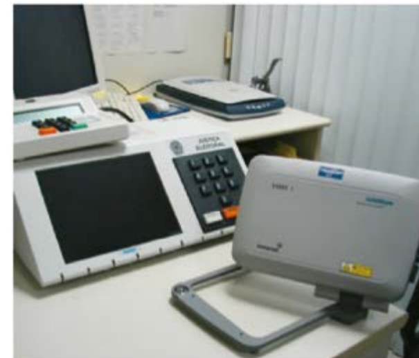
BGAN terminals like this one transmitted results gathered by electronic voting machines
